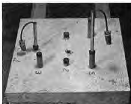
Fig. 6—Specimen with Menzel's device installed
