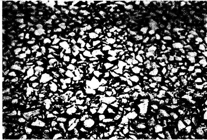
Photo 5—Open permeable texture of O.G.D.L.
