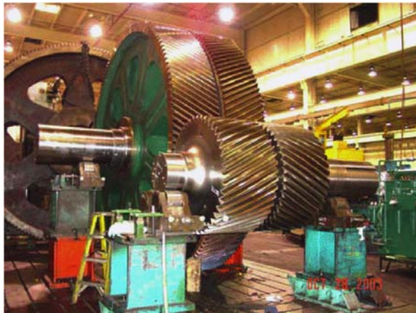
Figure 5. Typical Large Rolling Mill Gear Set
