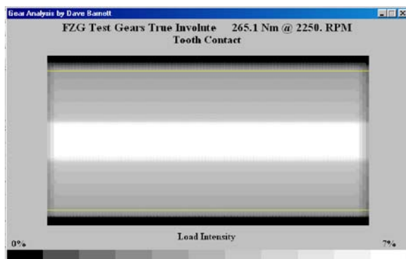
Figure 2. Load Intensity - Standard FZG Test Gear
