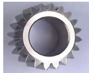
Figure 1b. Planetary gear of a reduction unit in a Scania heavy truck gearbox.
