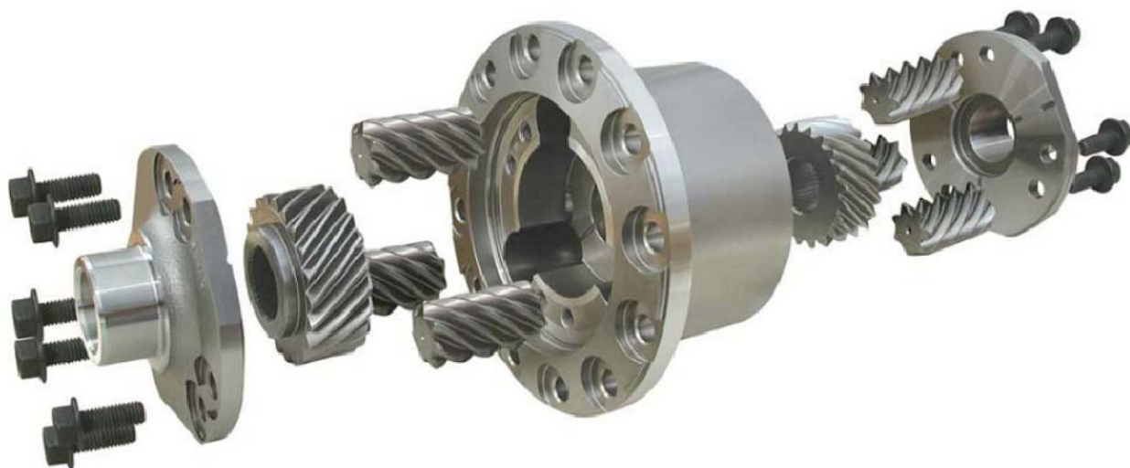
Figure 1. An example of application of helical STN -gears [2], [3].
