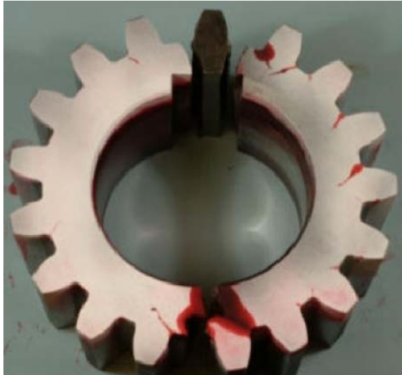
Figure 3 - Failed Final Drive Spur Pinion
