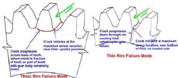
Figure 4 - Comparison of Thick and Thin Rim Failure Modes
