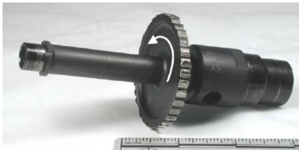
Figure 4. Failed spare drive gear
