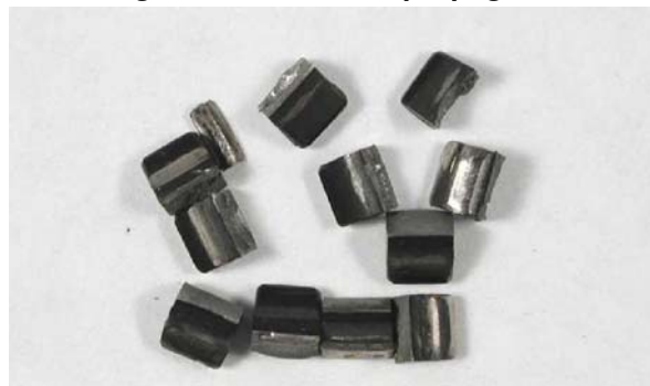
Figure 6. Condition of detached spare drive gear teeth
