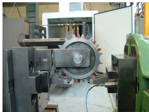
Figure 4. Fixture designed for AgustaWestland tests
