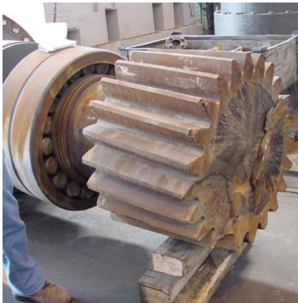
Figure 1. Large mill gear failure (note leg at left for scale)
