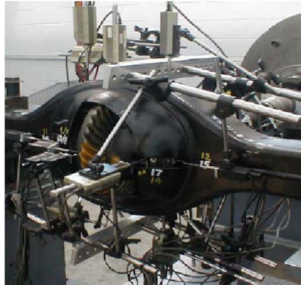
Figure 3. Experimental measurement of an axle deflection
