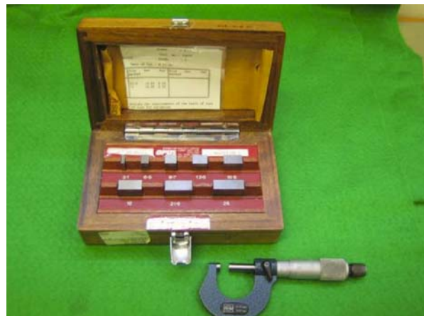
Figure 3. Micrometer and M8 gauge block set used for functional micrometer calibration
