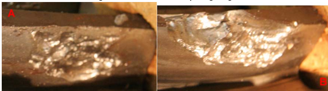
Figure 3. Heavy pitting often leads to local tooth fracture
