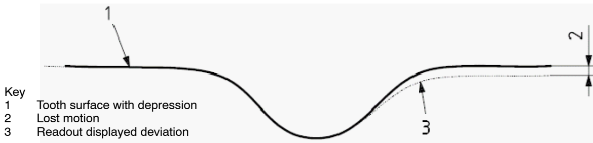
Figure 14 - Gaging system lost motion
