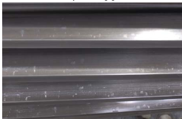
Figure 1c. Foreign object debris (FOD) damage
