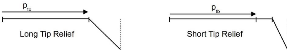
Figure 5. The extent of long and short tip relief
