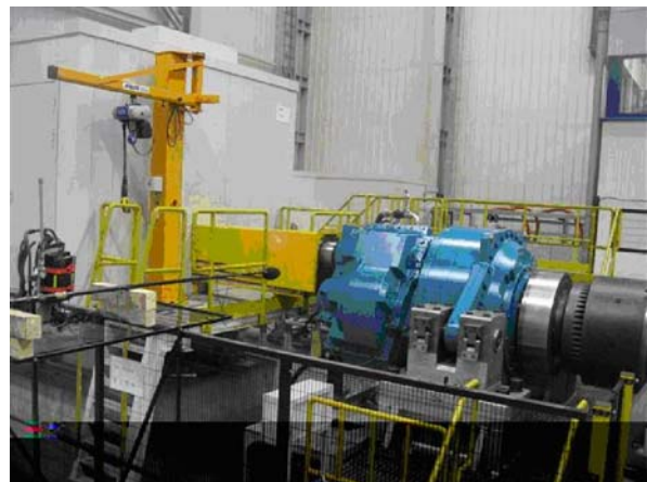
Figure 4. Gearbox on back-to-back test rig
