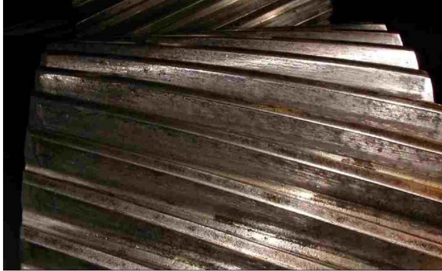
Figure 3. Wear on an industrial gear
