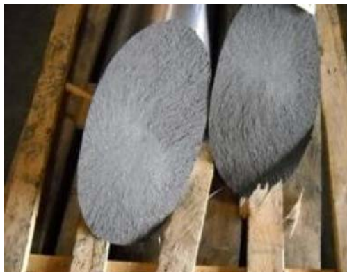
Figure 3. Sudden breakage due to hydrogen embrittlement
