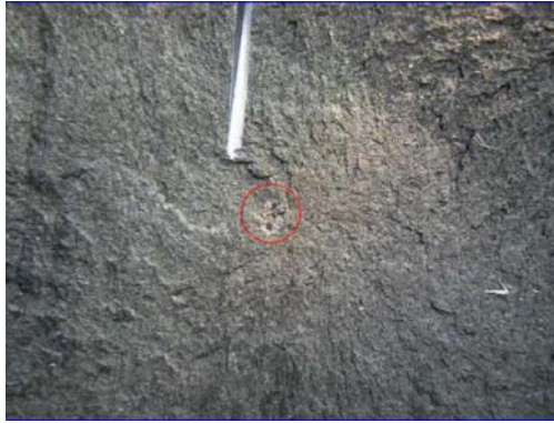
Figure 4. Magnification of hydrogen burst in the broken surface
