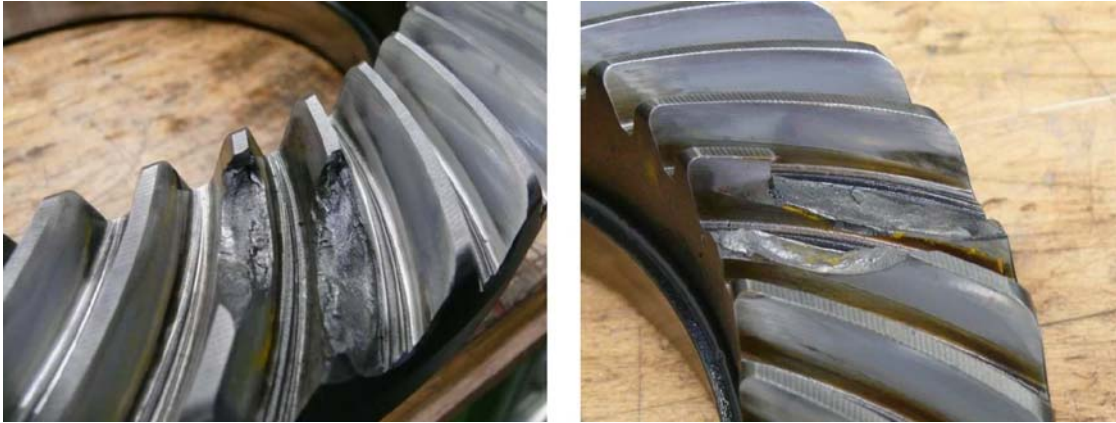
Figure 2. Flank breakage on two different wheels
