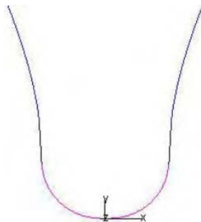
Figure 3. Trochoidal root profile
