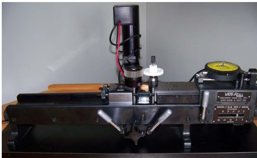
Figure 2. An actual double flank composite tester in tight mesh (Courtesy of Web Gear Services Ltd.)
