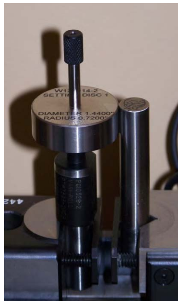
Figure 4. Calibration for tight mesh center distance (Courtesy of Web Gear Services Ltd.)
