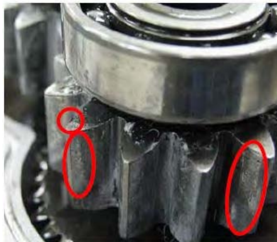
Figure 6. Damaged gear without crowning [7]
