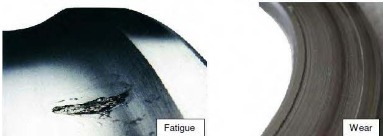
Figure 5. Typical rolling bearing failures
