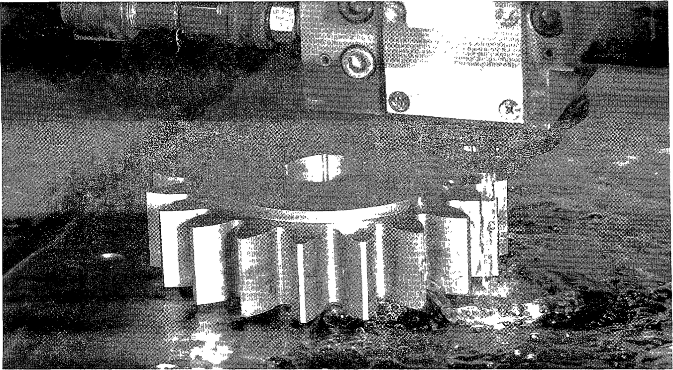
Figure 1 - Wire EDM gear cutting setup
