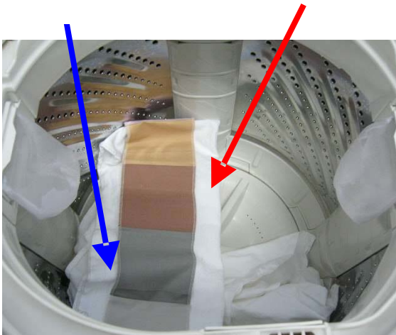
Figure 8 – Vertical axis washing machine: placement of items in the drum
