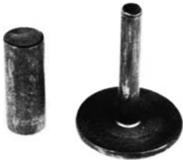
Figure 8. Shank of this part was extruded, and the head upset, to produce the exaggerated head to shank
