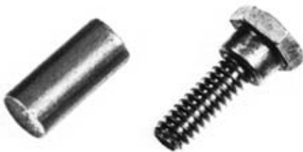
Figure 9. The shoulder on this part is the same size as the wire diameter, while the shank was extruded and the head upset.
