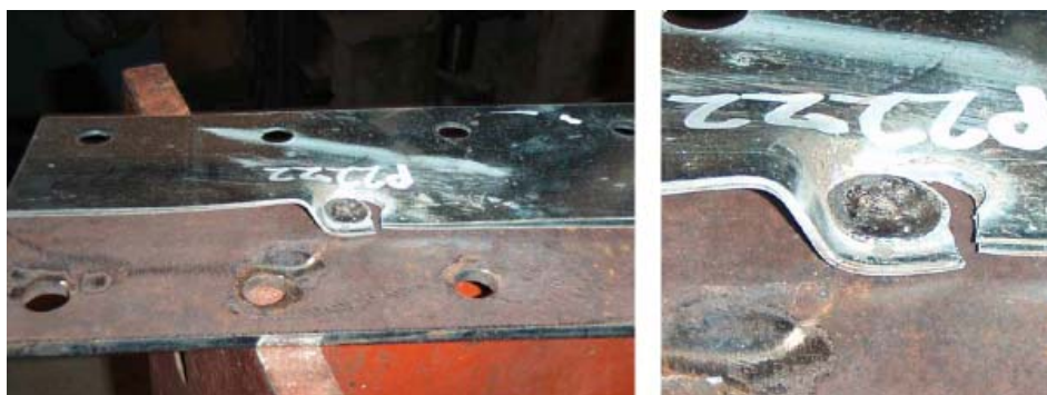
Figure 1.4: Sheet tearing failure mode (Guenfoud, 2010).
