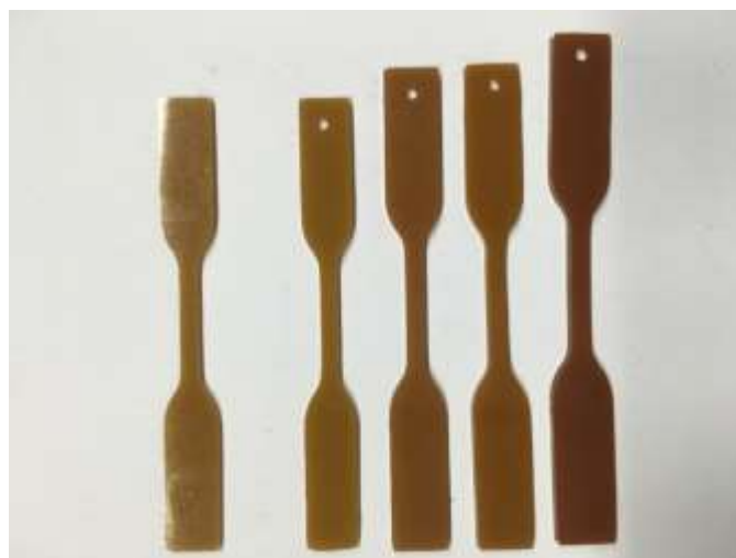
Figure 1: PUR after 84 days exposure at 40 °C, from left to right: reference, without media, B0, B20 and aged B10
