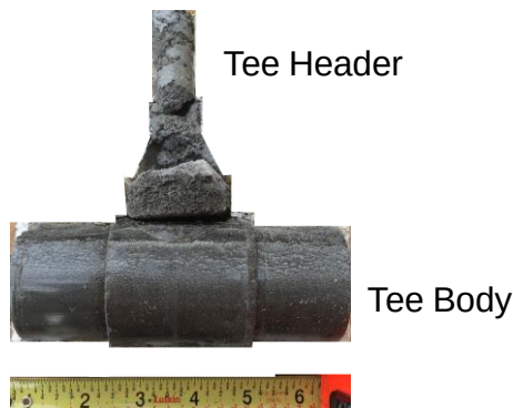
Figure 3: Example of deficient grout in the INT.
