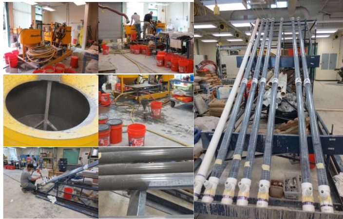
Figure 2: Example of the modified incline tube test.
