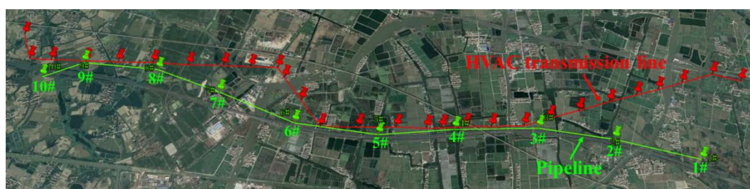
Figure 1: Pipeline and HVAC transmission line route
