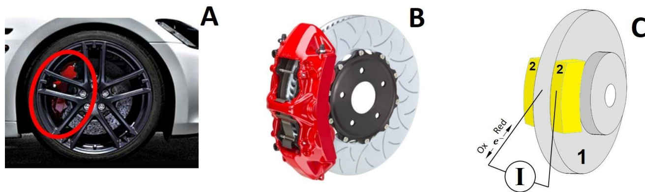
Figure 1: A) Car wheel comprising a disc brake system; B) Disc brake system for high end cars; C) Schematic illustration of disc (C1) and braking pads (C2); the galvanic current (I) between the two and the associated electron flow are represented by the means of black lines. Considering the used experimental setup, oxidation of the disc is associated with positive currents while negative currents are associated with the oxidation of friction material comprised in the braking pads.
