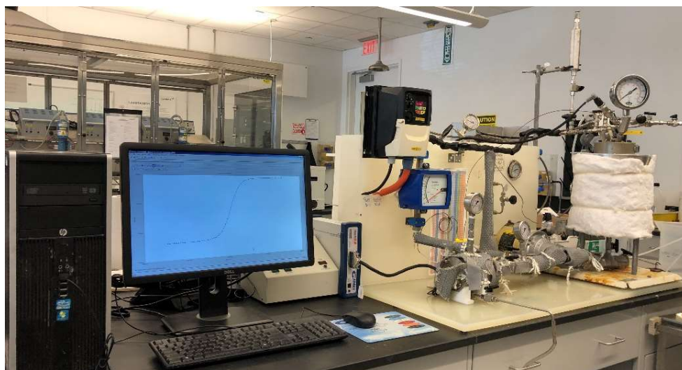
Figure 3: Jet Impingement system for high shear testing
