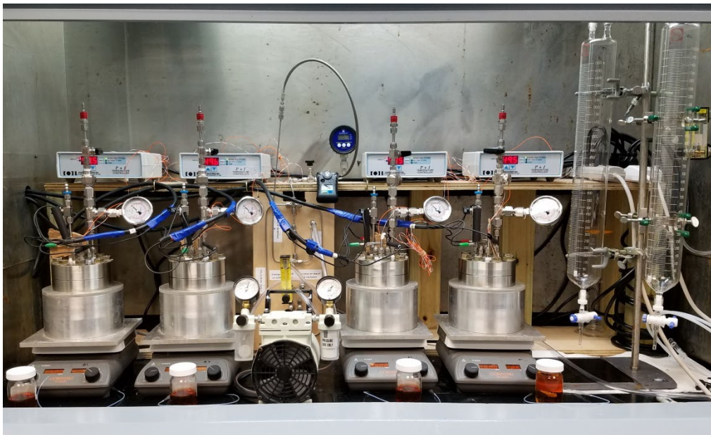
Figure 1: Electrochemical Autoclave Setup
