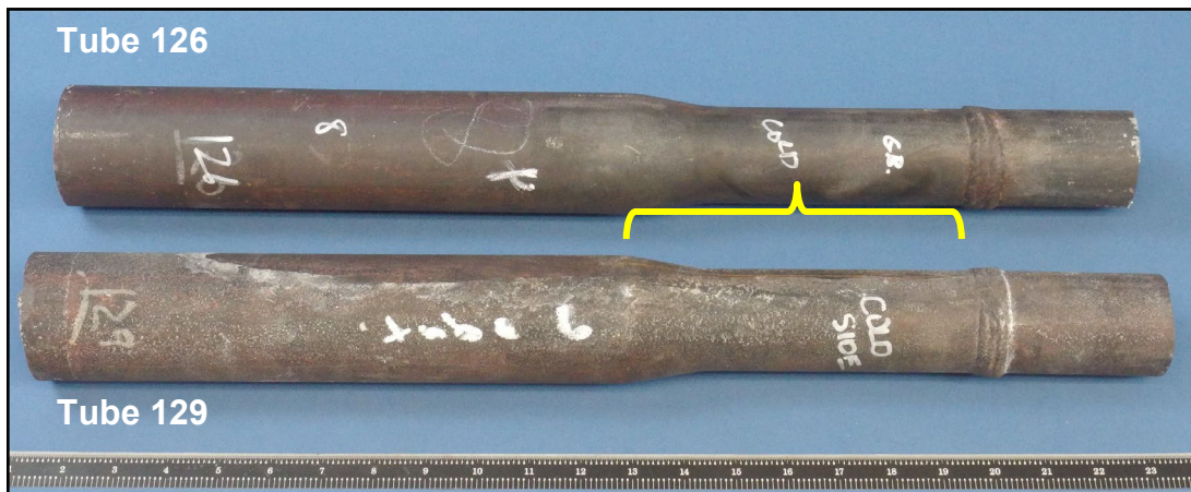
Figure 2: Screen tubes received for analysis. Bracket indicates crack location.
