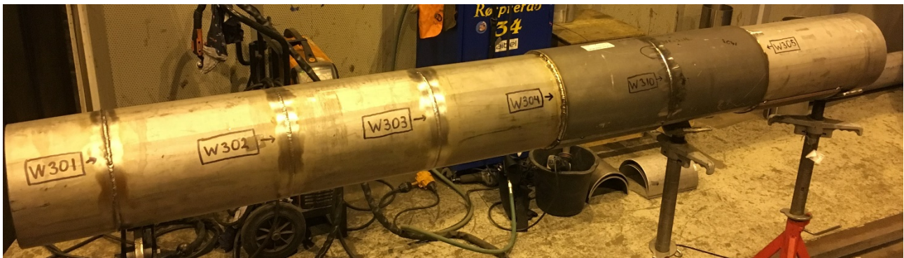
Figure 2: Test spool 3 after completion of all welds. Each weld identified by weld numbers.
