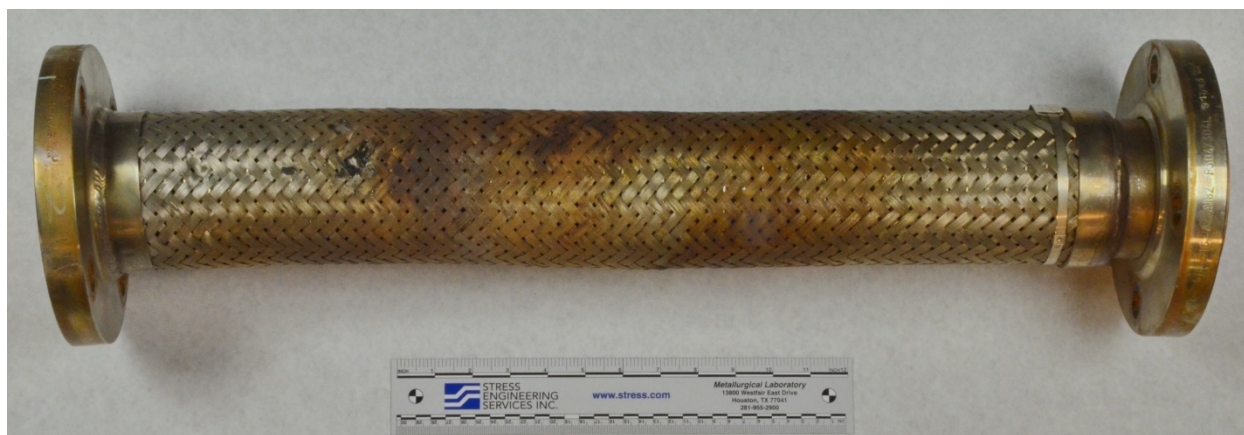
Figure 1: Leaking fuel gas 304L flex hose as received for analysis. Numbered scale divisions are inches/cm.
