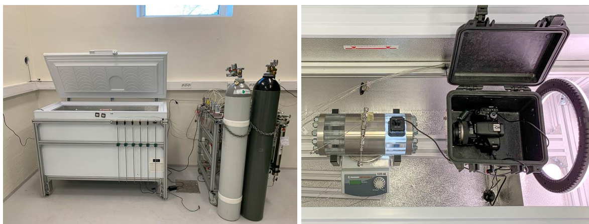
Figure 1: Picture of the test system (left) and picture inside cooling chamber with transparent autoclave, tubing, camera and LED light (right).
