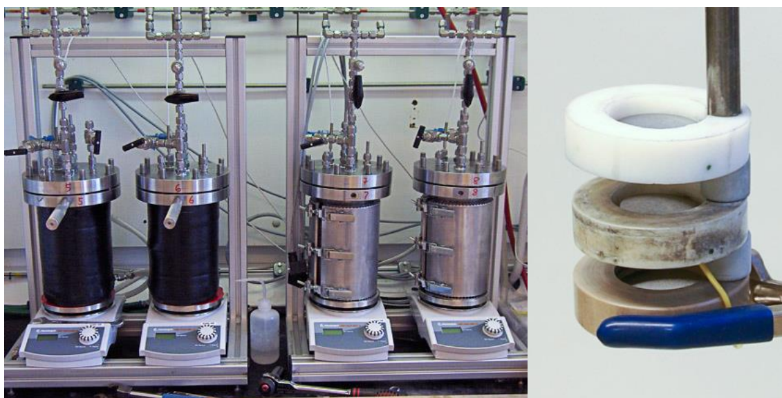
Figure 2: Hastelloy autoclaves (left), sample holder with coupons (right).
