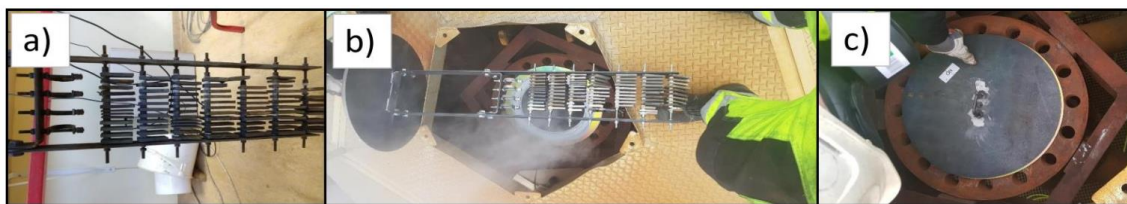
Figure 2: Test A – Wellhead, a) Coupon samples in a testing rack, b) install of coupons in wellhead and b) coupon samples inserted in wellhead (Courtesy of ON)
