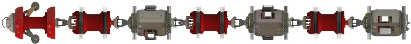
Figure 3: Image of the 10-inch EMAT tool configuration used for validation.
