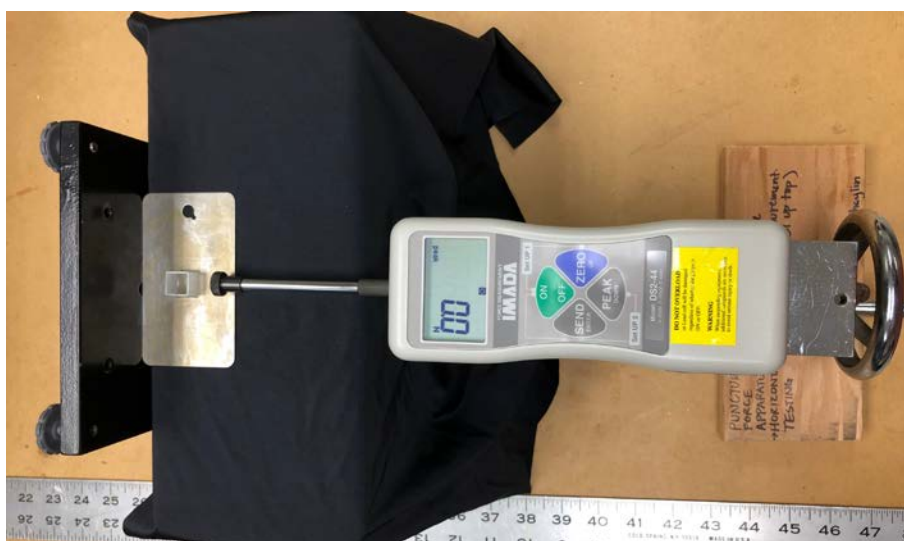
Figure 1 – Apparatus for testing wax adhesion to various metal surfaces.
