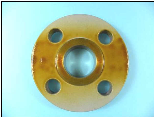
Figure 2b: Appearance of Flange Face with Rust Preventive Coating
