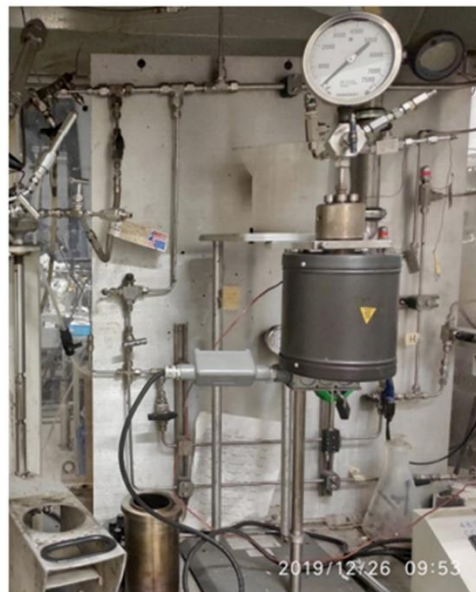
Figure 1: Schematic diagram and a photo image of the 75 mL batch-mode SCWG reactor setup used in this study
