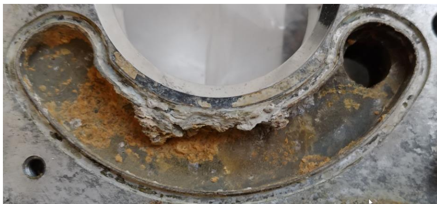
Figure 1. Corroded aluminum mold from plastic molding production. The metal is Al7075.
