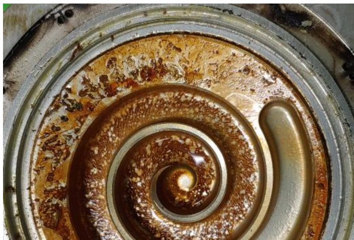
Figure 2. Aluminum mold from a bottling plant. The mold is made with aluminum alloy 6063.
