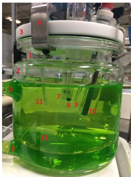
Figure 2. A picture of the custom-made glass cell and its components used in the RDE electrochemical experiments: (1) glass cell, (2) outer jacket, (3) Teflon lid, (4) clamp, (5) coolant (glycol) in, (6) coolant out, (7) RDE and its holder, (8) pH probe, (9) Luggin capillary for the Ref. electrode, (10) counter electrode, (11) thermocouple, and (12) magnetic stirring bar.
