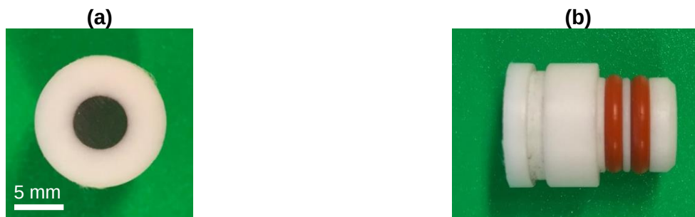
Figure 3. (a) The bottom view of the RDE specimen flush mounted in a Teflon holder, (b) The side view of the specimen holder.
