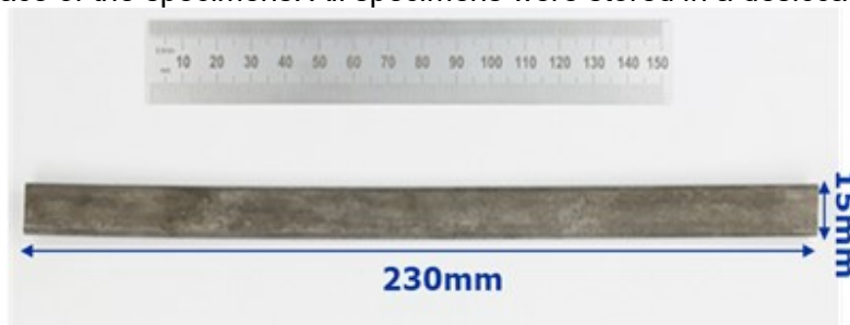
Figure 1: Images of the test material after cleaning as per BS ISO 8407:2014 standard, prior testing for tests in current study
