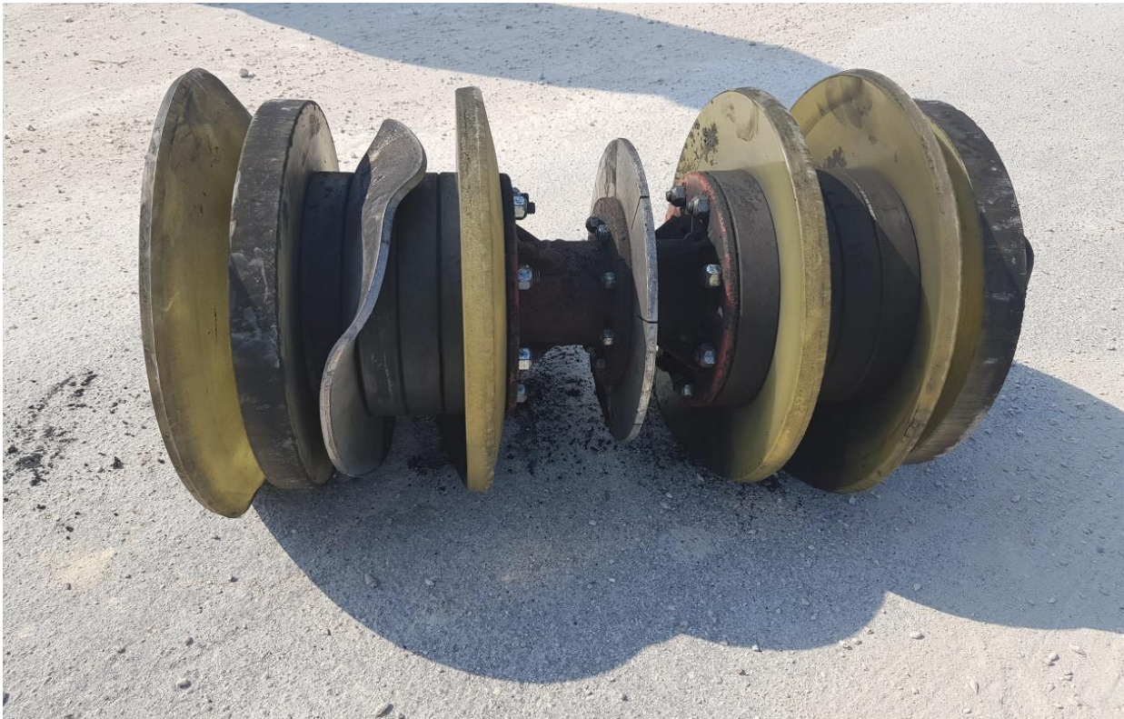
Figure 2: Gauge plate after passing through 14inch diameter pipeline damage due to half open valve
