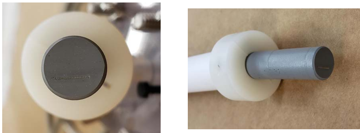
Figure 2: Photographic image of the MEA probe: (a) end view showing the 20 AA7075 wires and (b) a side view showing the mounting assembly.
