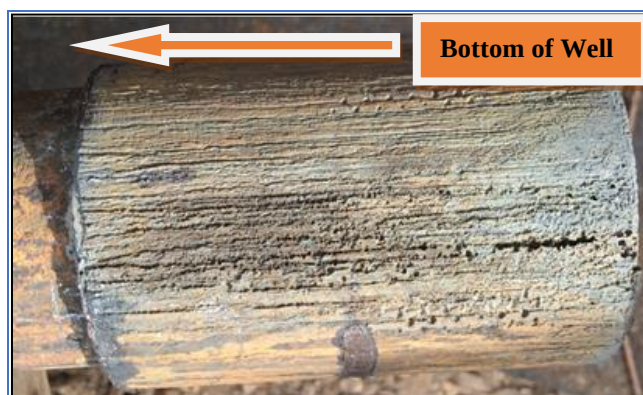
Figure 1: Imprints on production-tubing collar by direct contact with scale products for months
